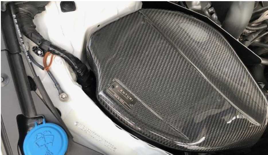
19. Locate it into the 2 mounts and press firmly into place.
