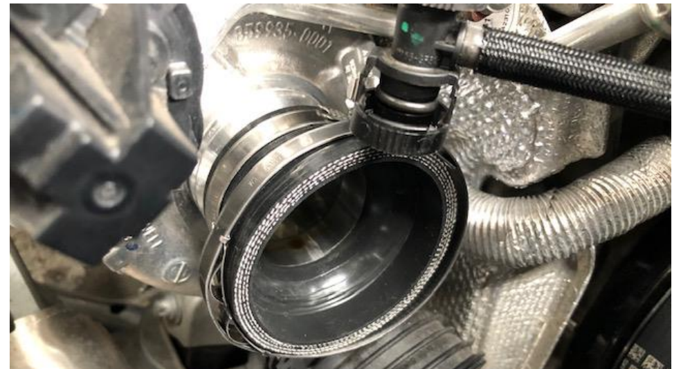
8. Push the provided silicon reducer onto the turbo with the 2 clamps. Secure the turbo side clamp.
