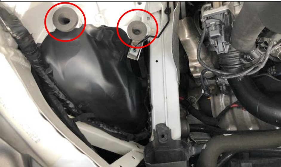
7. Remove the tube completely. Make sure the rubber mounts are in place.
