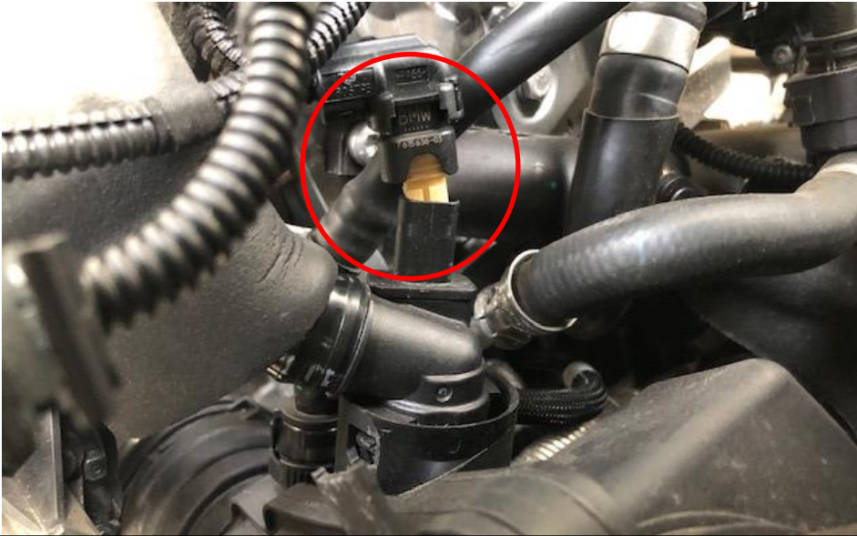
5. Disconnect the plug on the inlet tube near the turbo.
