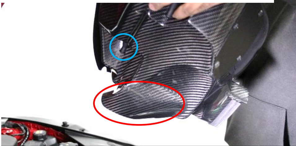
13. Carefully lower the airbox into the engine bay. Note that the secondary scoop circled above goes into the gap shown in the next photo. Also the mount circled blue should sit in the rubber mount shown in next photo.
